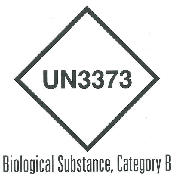
Do NOT resize or rotate these labels. Attach labels to a vertical side of the box (not the top or bottom). Each diamond must be 4" x 4" large, "square-on-point",  $\geq$ 3 inches away from other markings that may reduce its effectiveness.
