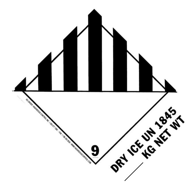
Do NOT resize or rotate these labels. Attach labels to a vertical side of the box (not the top or bottom). Each diamond must be 4" x 4" large, "square-on-point" with the #9 at the bottom, <u>>3</u> inches away from other markings that may reduce its effectiveness. NOTE: USPS will not transport dry ice, use UPS or FedEx.
